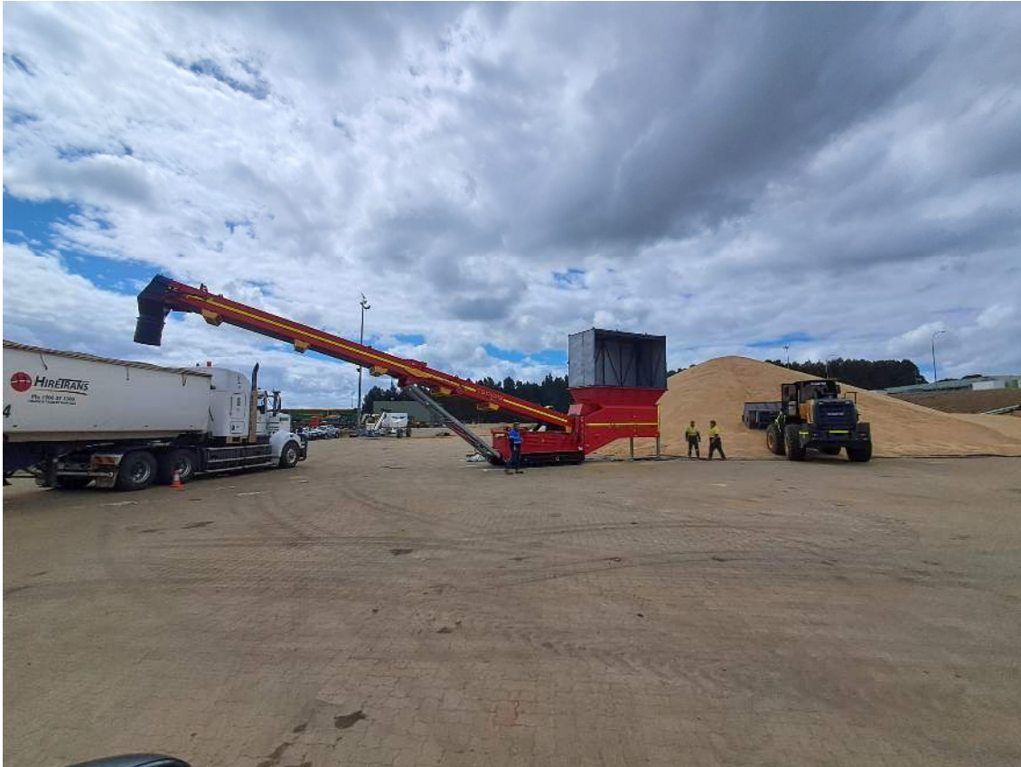
Figure 7 Mobile Conveyor in Operation Offloading Grain from a Stockpile
