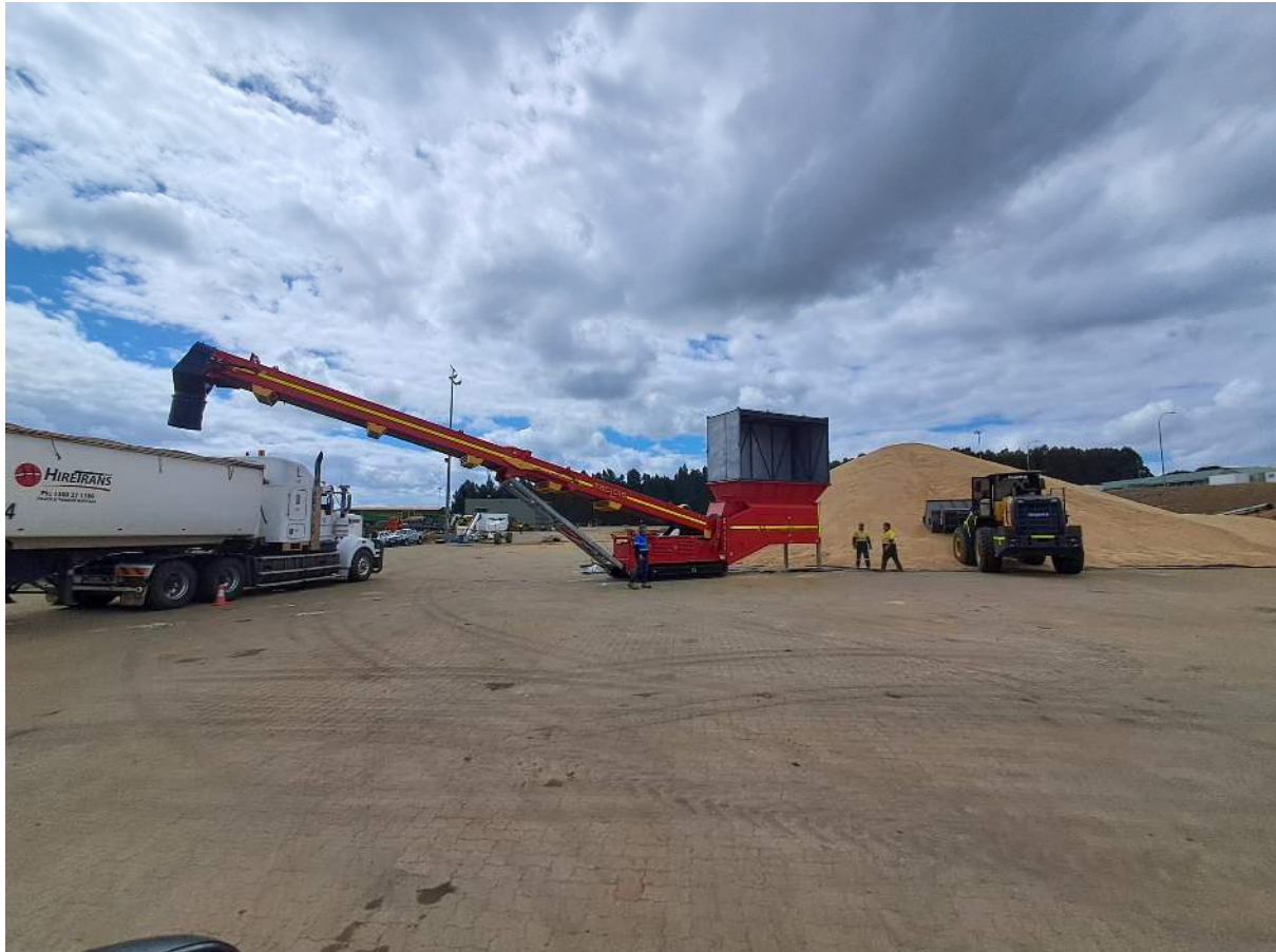
Figure 1 Mobile Conveyor in Operation Offloading Grain from a Stockpile (see also separately provided video)
