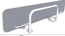
Raise the side safety rail when the person has been placed on the table. Swivel side rail into position until the latch 'clicks' into position. Test side rail is secure.
